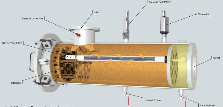
Dirt Defence Filters are designed to remove fine solids such as rust, sand and other particulates efficiently and continuously from aviation fuels. Dirt Defence Filtration Technology in combination with AFGUARD<sup>®</sup> Electronic Water Sensor has become a global norm (JIG 1 and ATA 103).
