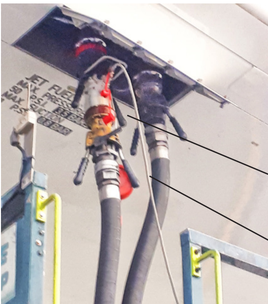
Biocide Hydrant Coupler connected to an Aircraft
